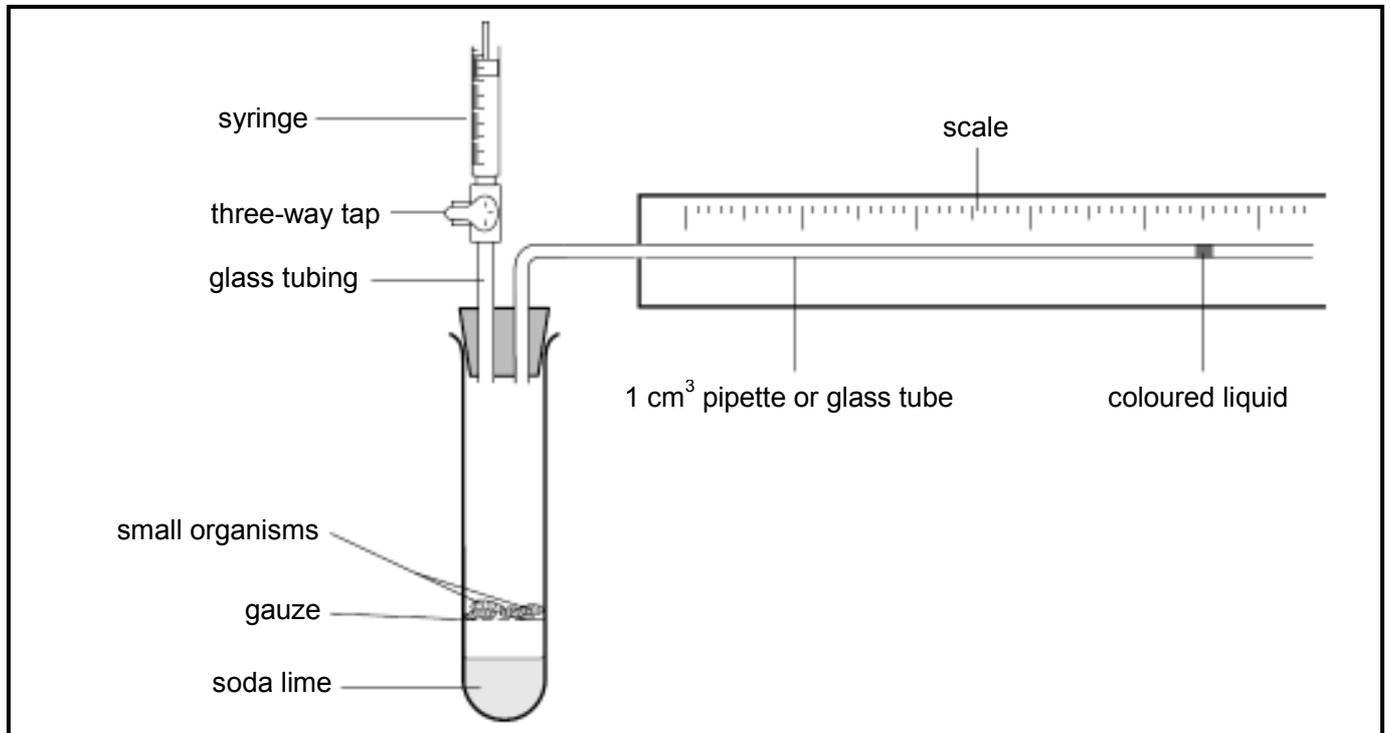
Figure 1 A simple respirometer using a boiling tube
