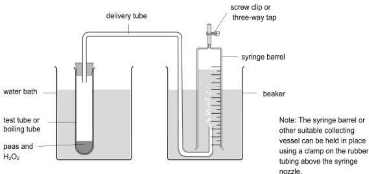
4. Place the boiling tube in a waterbath at  $20^{\circ}C$  to acclimatise
