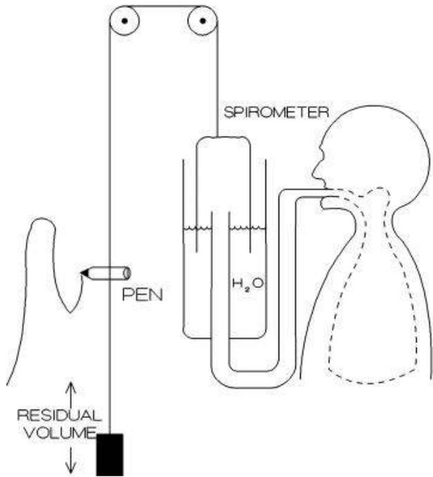
A simple diagram of a spirometer
